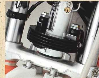
Compact, high efficiency oil cooler mounted on steering head stabilizes engine temperatures.
