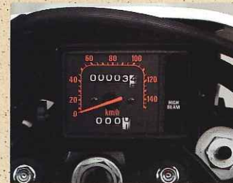
Enduro-type speedometer and set/trip meter illuminated for high visibility.
